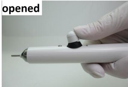
Now insert the tool as far as possible. Pull back the black knob and the tool will be clamped.
