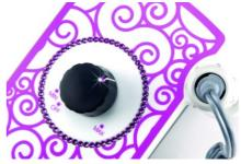
The handpiece only starts at minimum speed. By turning the button more in a clockwise direction, you will raise the speed.
