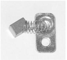
Put in a new carbon brush. Check the position of the spring on the brush. It must be in the middle of the brush. The carbon brush is a wearing part and has to be exchanged when worn. You will find a pair of carbon brushes enclosed. Check the second brush as well.
